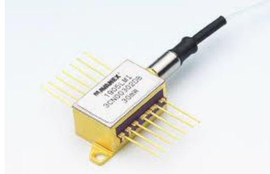
Fig. 2. DFB laser module A1905LMI.
